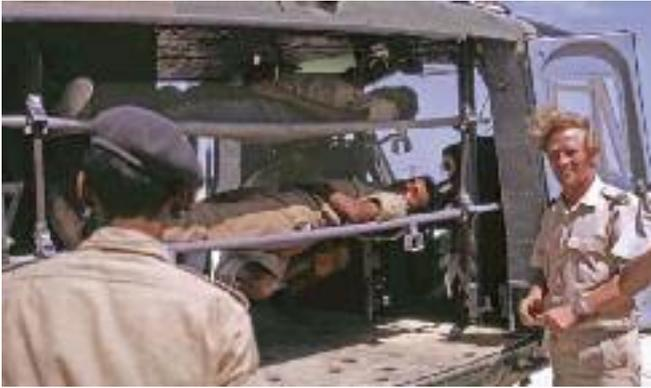
Fig 2: The Huey set up to take six casualties. Three could be carried transversely with more space.
